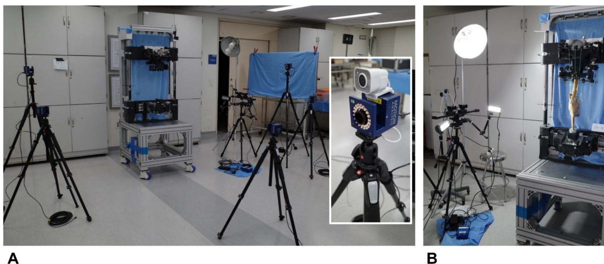
Figure 3. Biomechanical test setup. The motion capture system included five cameras; optical markers were placed when measuring knee kinematics (A). Real-time changes in MCL strain during flexion were analyzed using a noncontact video extensometer with a high-resolution digital camera and real-time image-processing software. A camera was placed 1 m from each specimen mounted in a customized knee-squatting simulator (B).
