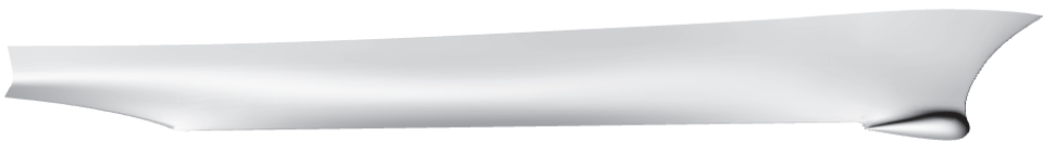
Figure 10. Schematic of a 3D model of DTMB 5415.
