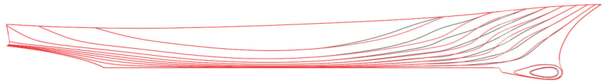
Figure 24. Comparison of profile views of hull forms obtained by direct and dimensionality reduction optimizations.
