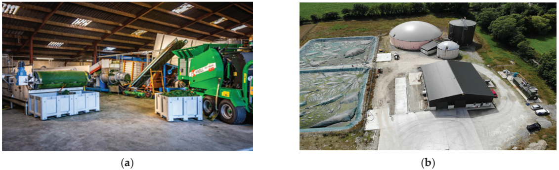
Figure 3. (a) Grassa 4-tonne per hour pilot green biorefinery plant production unit for LPC; (b) Timoleague AgriGen Biodigester for supply of slurry to produce biogas.
