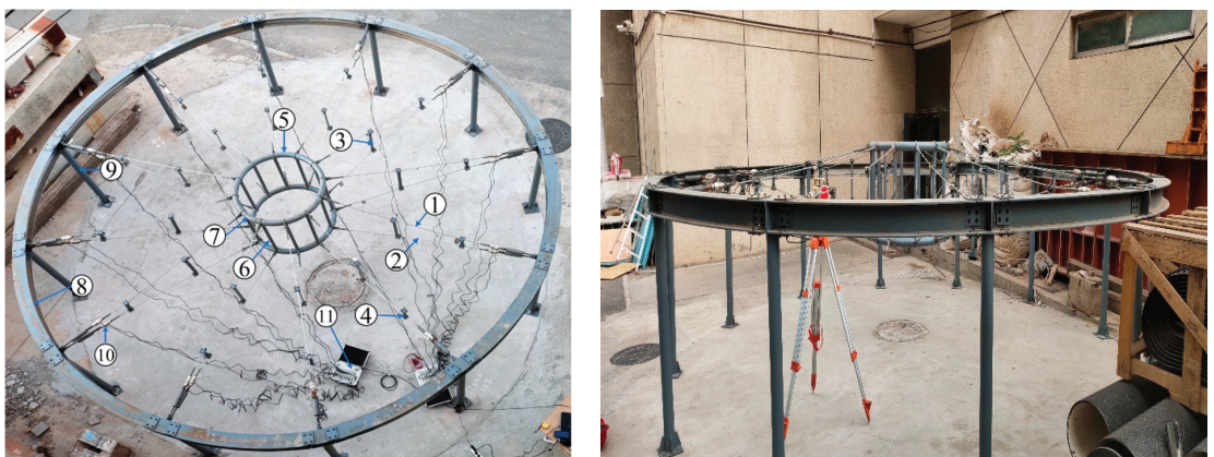
Figure 4. The experimental model: (① URC, ② LRC, ③ middle strut, ④ outer strut, ⑤ upper ring beam, ⑥ lower ring beam, ⑦ inner strut, ⑧ outer ring beam, ⑨ outer column, ⑩ tension meter, ⑪ collecting box).
