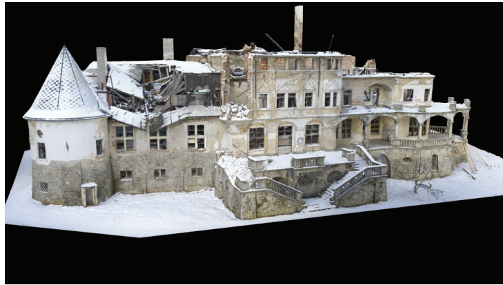
Figure 11. The Kunerad Castle model connected with terrestrial and aerial photogrammetry.
