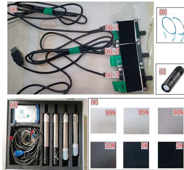
Figure 1. (a) Ocean Optics micro-spectrometers (STS-VIS); (a)-1 sensor for measuring sky radiance; (a)-2 sensor for measuring water radiance; (a)-3 sensor for measuring downward irradiance. (b) Ocean Optics and Hygirel fiber. (c) Cosine Correctors. (d) Trios. (e) Diffuse reflectance plates and target cloth (99%, 95%, 30%, 20%, 5%, and 2%).
