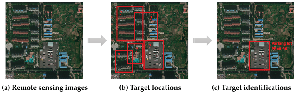
Figure 4. Target detection schematic. (a) is the original remote sensing image; (b) reflects that the candidate locations of the targets are found in the image; (c) reflects the results of target identifications.
