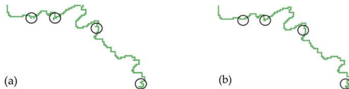
Figure 5. Contrast between before (a) and after (b) burr removal.
