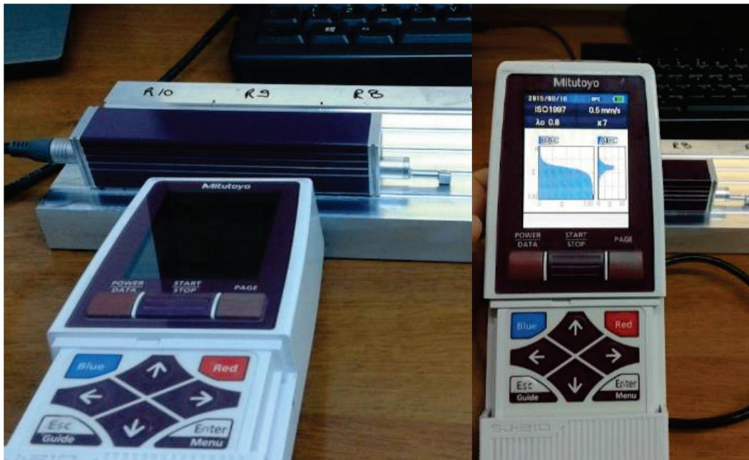
Figure 6. The measurements made with Mitutoyo SURFTEST SJ-210.
