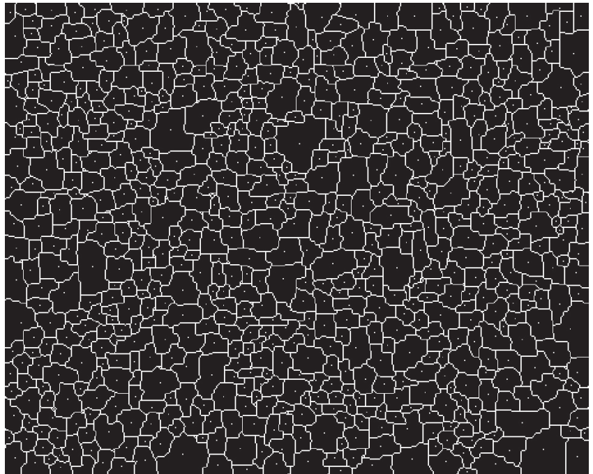
Figure 2. The multiresolution segmentation result and the centroids within each image object.
