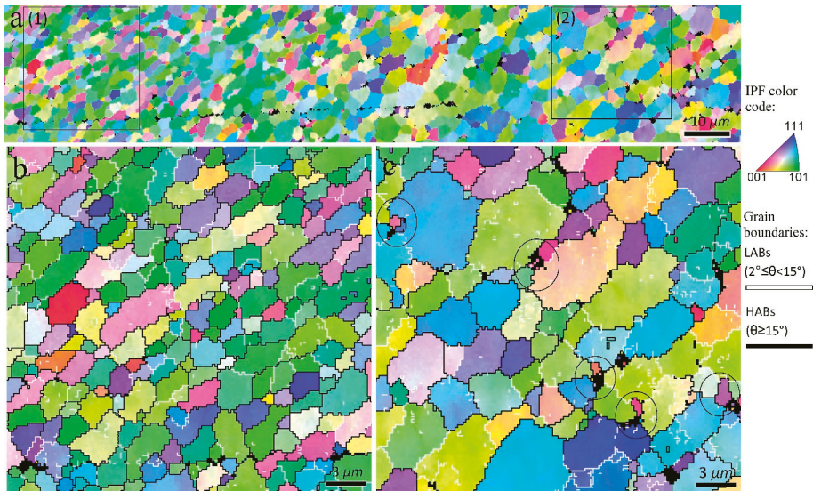
Figure 11. Inverse pole figure maps of the interfacial area between TMAZ and SZ-II in the 3-pass sample indicated by rectangle 1 in Figure 10. Higher magnification of zones 1 and 2 indicated in (a) are illustrated in (b,c), respectively. The circles in (c) refer to the non-index regions containing fine DRX grains, i.e., particle stimulated nucleation mechanism.
