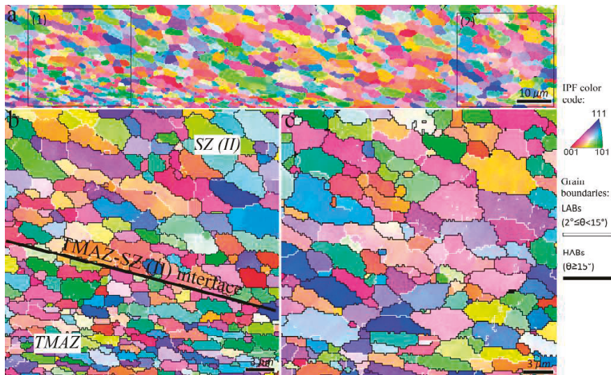
Figure 9. Inverse pole figure maps of the area indicated by rectangle 2 in Figure 7. Higher magnification of zones 1 and 2 indicated in (a) are illustrated in (b) interfacial area between TMAZ and SZ-II and (c) SZ-II, respectively.
