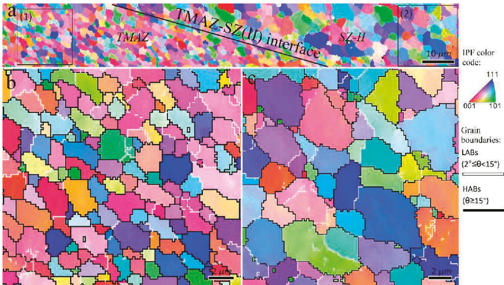
Figure 5. (a) Inverse pole figure maps of the interfacial zone between TMAZ and SZ-II regions in 1-pass sample indicated by rectangle 3 in Figure 2b. (b,c) Higher magnification of zones 1 and 2 indicated in (a), respectively.
