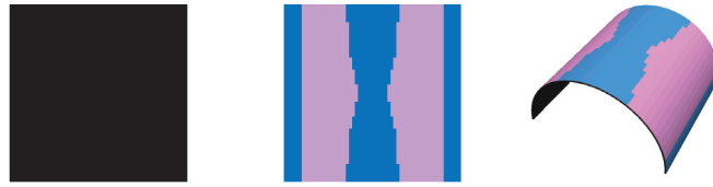
Figure 2. Structure layout \rho_s (left), electrode profile \rho_p (centre) and 3D design (right) for the first example.
