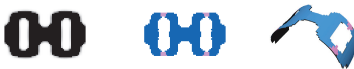
Figure 3. Structure layout \rho_s (left), electrode profile \rho_p (centre) and 3D design (right) for the second example.
