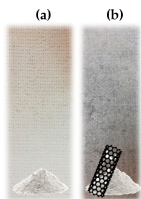
Figure 7. The image of photocatalysts: (a) TiO 2 photocatalytic film on glass fiber mesh, (b) TiO 2 /CNT photocatalytic film on glass fiber mesh.
