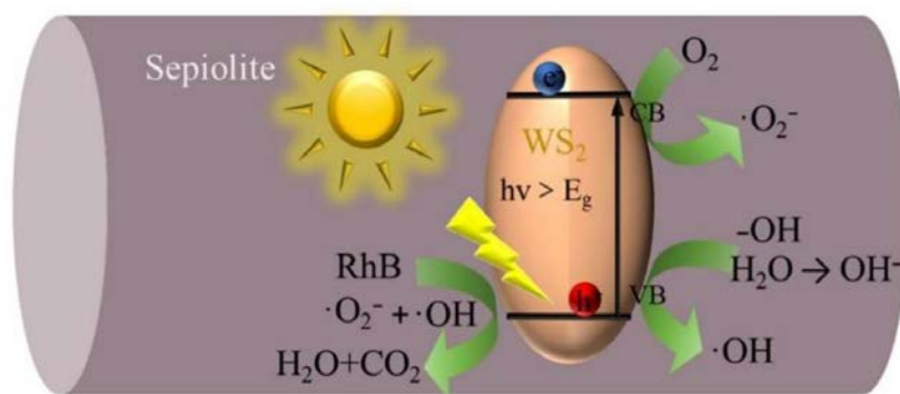
Figure 6. Possible RhB degradation mechanism of the WS 2 /Sep composite.
