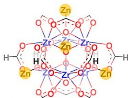
Figure 20. Zn-Zr cluster in the MOF-808-Zn catalyst for CO 2 hydrogenation (Zhang J. et al., 2021) [197].
