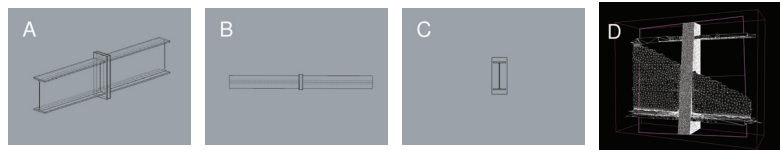
Figure 3. (A) The I-beam IPE400 with a thermal break in parallel perspective projection. (B) Top view. (C) Right view. (D) Section of the tetrahedral mesh.
