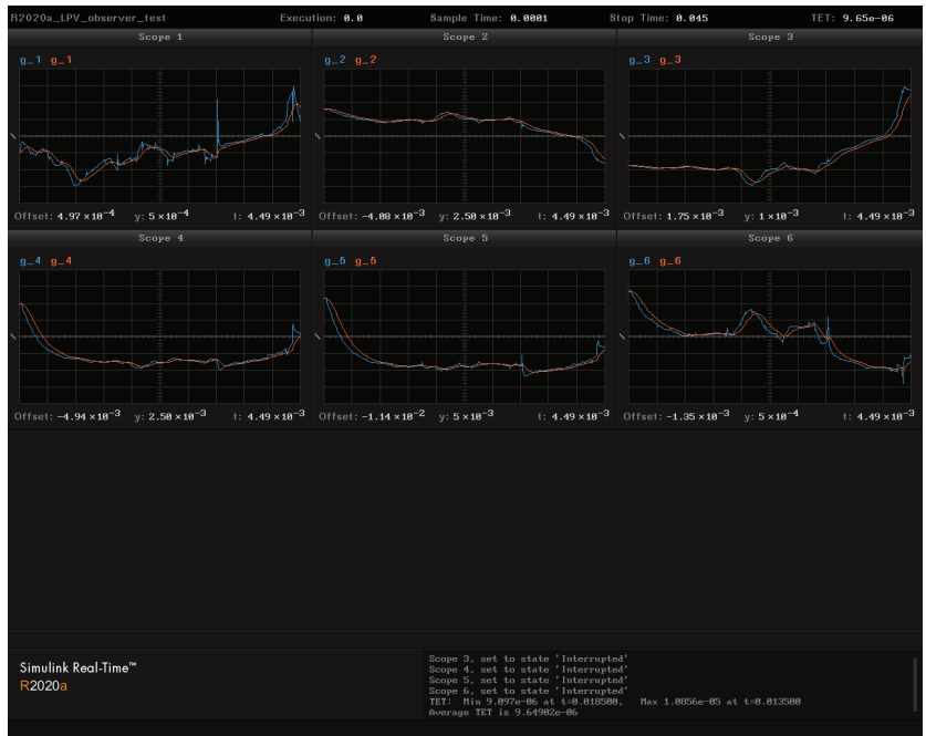
Figure 16. Real-time simulation of gaps variations \delta g derived by LPV model obtained from the FCDI code (blue line) and estimation of gap variations \delta \hat{g} obtained from robust observer synthesized by LMs (red line). Discharge #37263.
