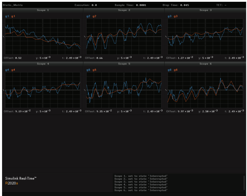
Figure 17. Real-time simulation of gaps g derived by LTI model obtained from the FCDI code (blue line) and estimation of gaps \hat{g} obtained from static matrix (red line). Discharge #37263.
