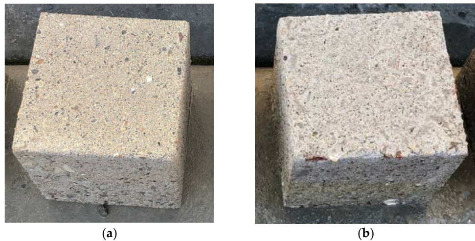
Figure 14. Concrete sample after acidic exposure for 28 days: (a) geopolymer, (b) OPC.
