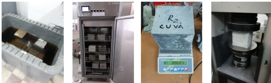
Figure 1. Control specimens kept in water and specimens underwent the freeze–thaw test (150 mm × 150 mm × 150 mm).
