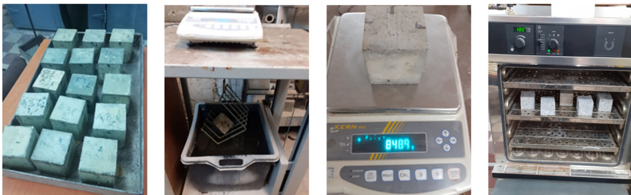
Figure 3. Hydrostatic weighing of cubes with 71 mm side.
