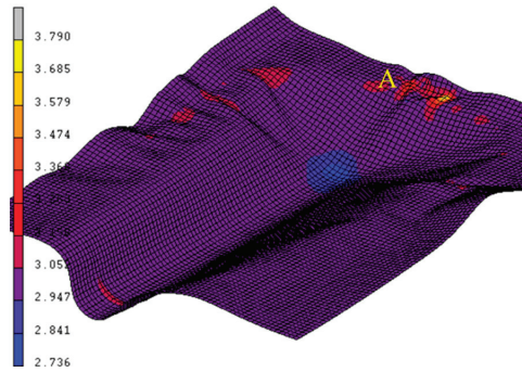
Figure 10. Thickness distribution of the drawing in the preforming process by the optimized design.
