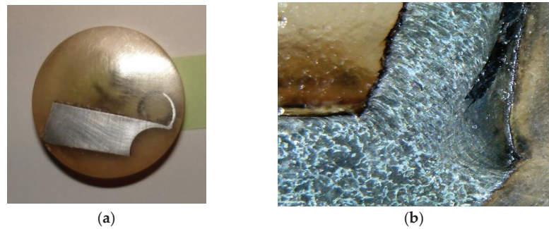
Figure 5. Investigated sample of a chip, (a) ground and polished, (b) etched, magnified 200 \times .
