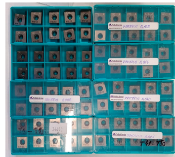
Figure 6. (a) Geometrical and dimensional characteristics of artificial wear; (b) Cutting inserts with prepared artificial wear.
