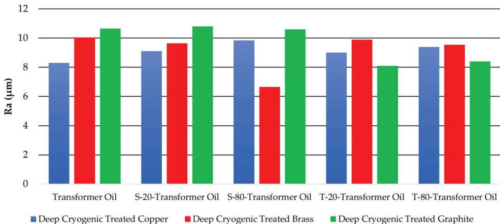
Figure 12. Surface roughness comparison of distinct deep cryogenically treated electrodes.
