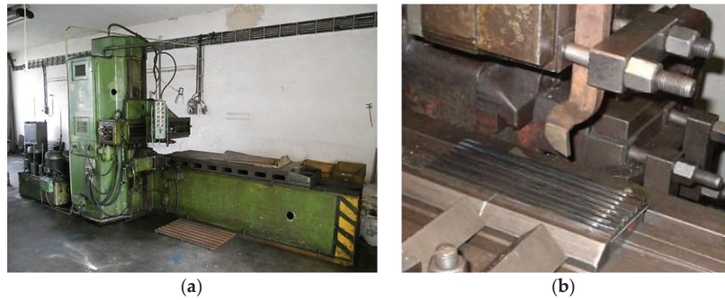
Figure 2. Experimental device (a) HJ8A planer, (b) experimental processing of a workpiece made of EN C45 steel.
