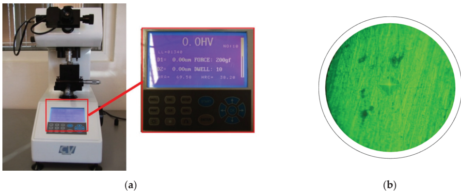
Figure 6. (a) Micro-Vickers hardness tester CV-403DAT; (b) tested samples—imprint, magnification 600 \times .
