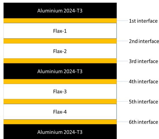
Figure 9. Schematic of interfaces between layers of the NFML.
