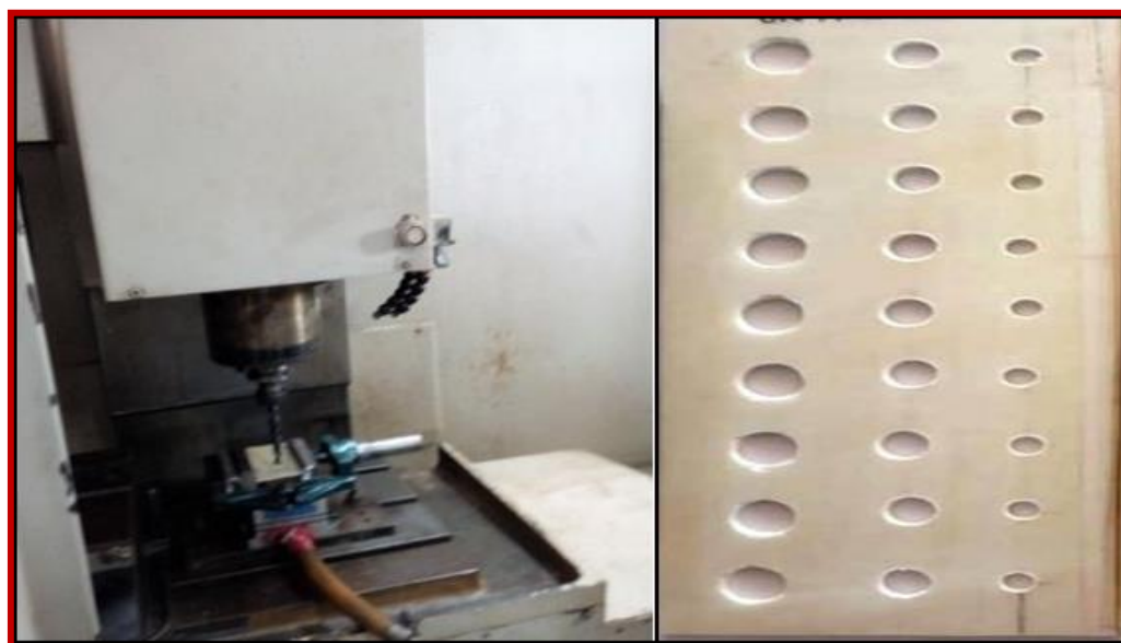
Figure 1. Drilling of CB composite laminate.
