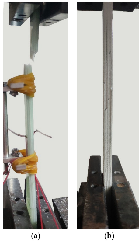
Figure 8. Tensile failure modes: (a) fiber fracture, and (b) delamination.
