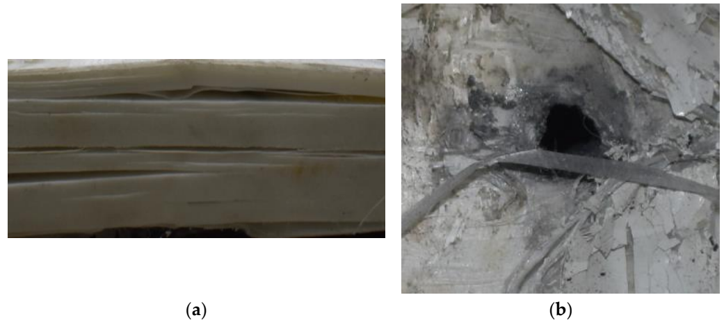
Figure 8. Failure states of the PE laminates. (a) Side view of PE laminates. (b) Outlet of PE laminate.
