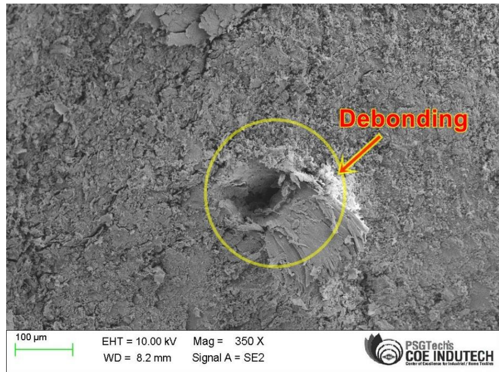
Figure 8. SEM image of drilled hole drill (2400 rpm and 20 mm/min).
