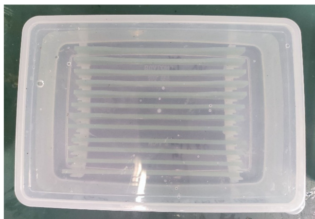
Figure 2. GFRP specimen immersion test.
