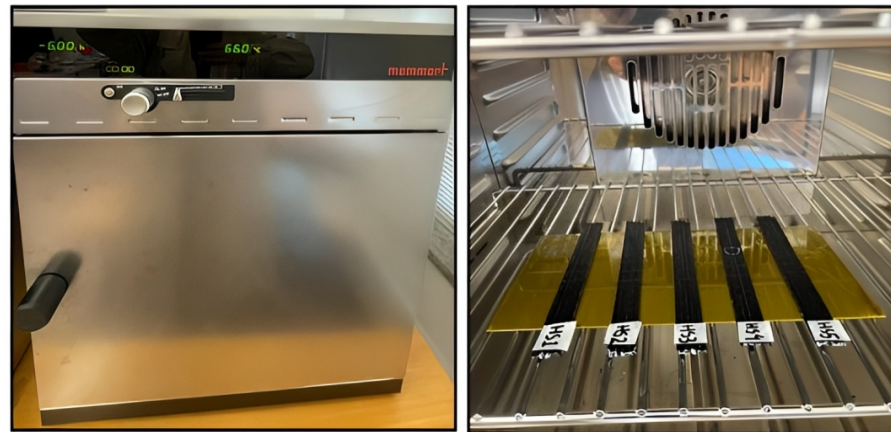
Figure 2. An air-circulated oven for hot temperature treatment.
