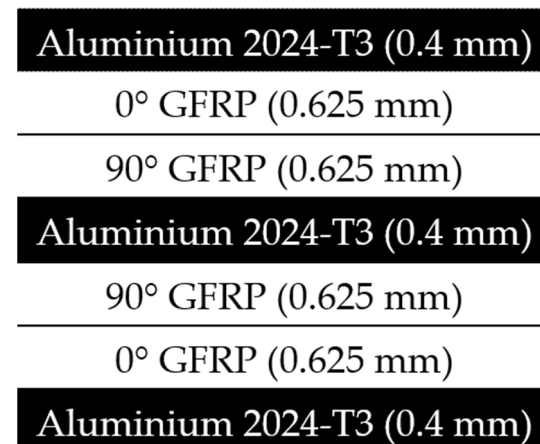
Figure 1. Schematic diagram of GLARE 3/2-0.4.
