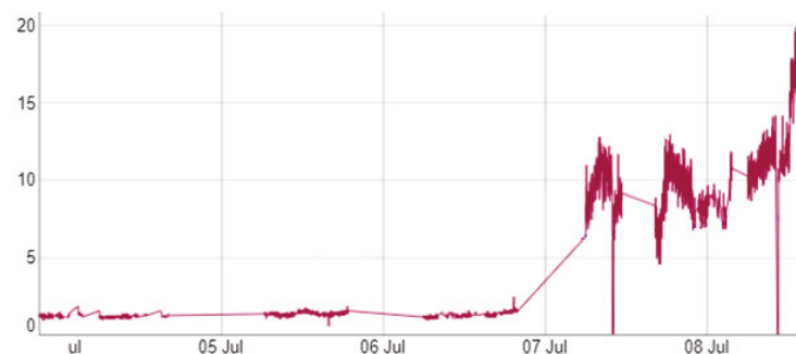
Figure 2. Change point of an elevator measured with a vibration sensor at the Ford factory located in Almussafes (Valencia).
