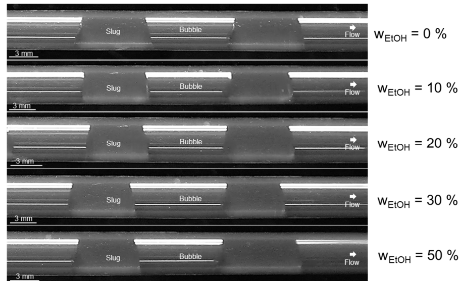
Figure 9. Depiction of the slug flow obtained in the experiments for evaluating the slug shape for different compositions of ethanol/water mixtures at a total volumetric flow rate of Q_{\text{tot}} = 20 \text{ mL min}^{-1} at ambient temperature ( \theta_{\text{amb}} \approx 22 \text{ }^\circ\text{C} ).
