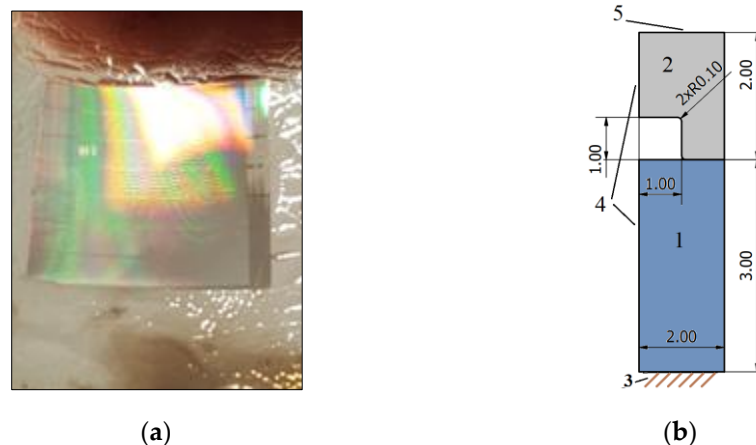
Figure 5. (a) Template of nickel master grating plate; (b) drawing of one master-grating element with boundary conditions: 1—substrate, 2—stamp, 3—fixed support, 4—symmetry region and 5—an external force.
