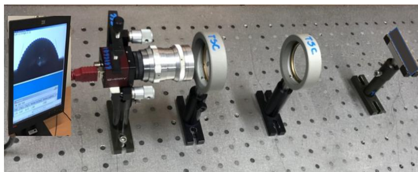
Figure 1. A contact angle measurement setup.
