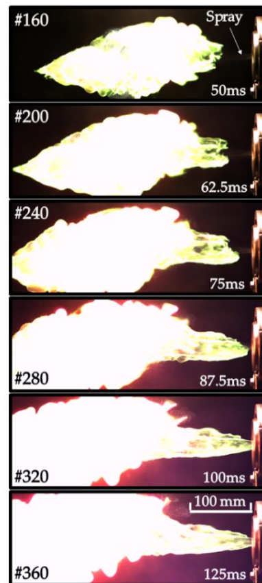
Figure 8. Sequence of video frames of continuous TEA–TEB spray combustion in ambient air at NPT conditions: recessed injector, the same test fire as in Figure 7. Injection overpressure is 3 atm. Frame size is 1280 \times 456 pixels ( 406 \times 145 mm 2 ), frame rate 3200 fps, shutter speed 300 \mu s, injection duration 500 ms.
