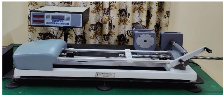
Figure 3. Electronic tensiometer for flexural and tensile properties testing.
