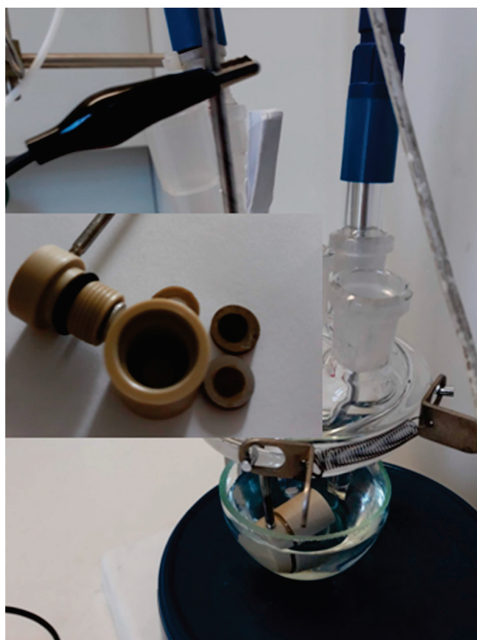
Figure 2. Electrochemical cell and disk work electrode.
