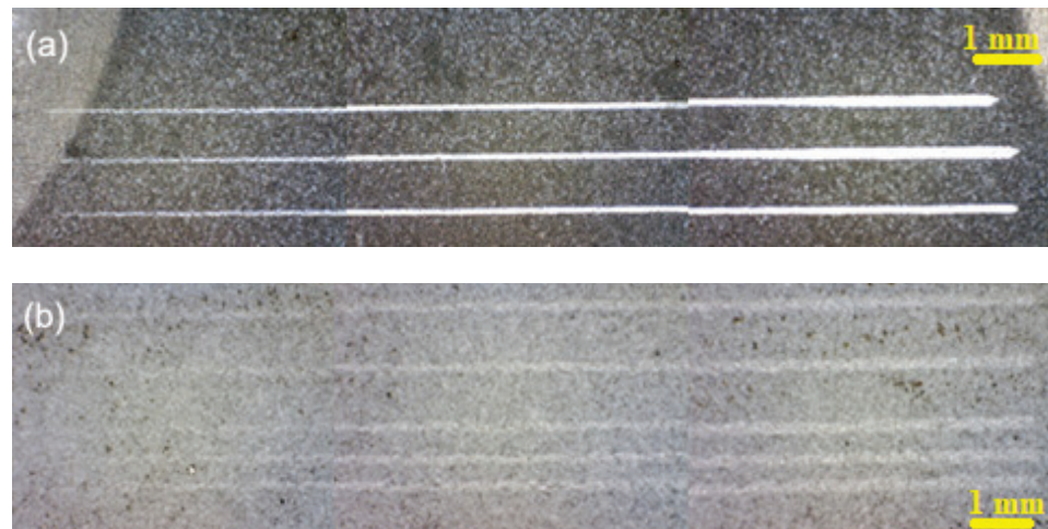
Figure 4. Identification and images of scratches using optical microscopy for the coatings: (a) two layers; (b) four layers.
