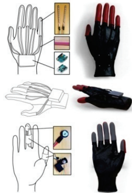
Figure 7. Prototype design of data glove based on emotion recognition of physiological signal.
