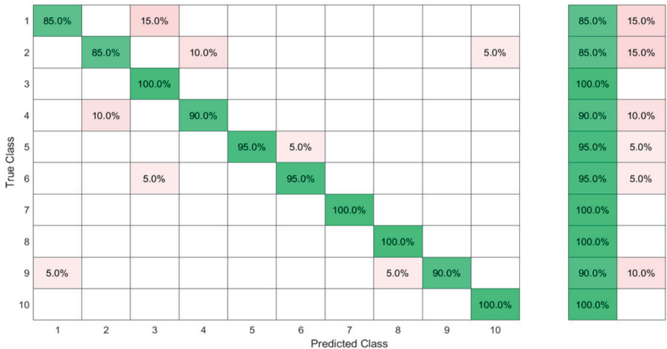
Figure 10. Ten ASL letters, A–J, detected with FMG and classified by the KTGEL.
