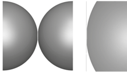
Figure 2. Treatment of contact points showing close-up views of caps approaches, for both particle-particle and particle-wall cases.
