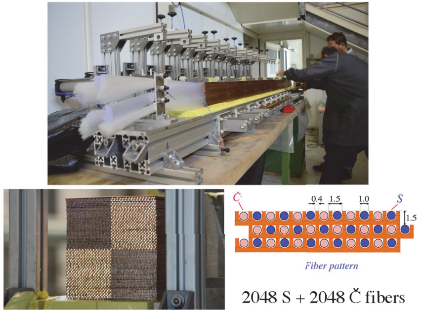
Figure 11. A fine-sampling copper-fiber calorimeter built by the Pisa group of the RD52 Collaboration.
