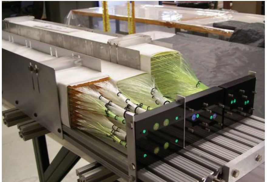
Figure 1. Three 105 cm long ADRIANO prototypes during the assembly phase at Fermilab's Thin Film Facility.
