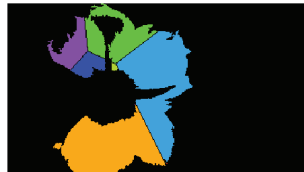
Figure 2. Voronoi area division of the bigger contour of the image of Figure 1b.
