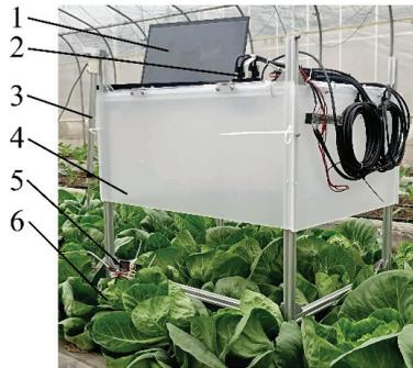
**Figure 14.** Accuracy test platform site. Key: 1. visual processing platform; 2. binocular camera with an 850 nm filter; 3. linear displacement sensor; 4. fixed support frame; 5. digital display for displacement sensor; 6. cabbage.
