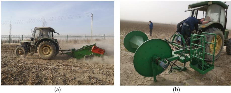
**Figure 8.** Test field of curl-up collecting of film. (a) 11SM-1.2 curl-up film collector; (b) 1JRM-2000 curl-up film collector.
