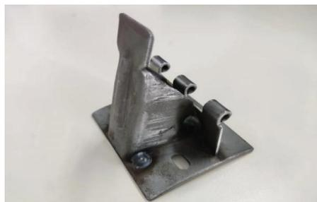
Figure 20. Welding forming of duckbill parts.
