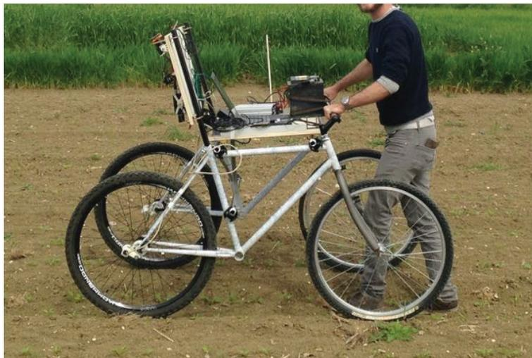
**Figure 4.** Acquisition process of the Sunflower dataset using a custom-built manual pushcart. Courtesy of Dr. Alberto Pretto—University of Padova.
