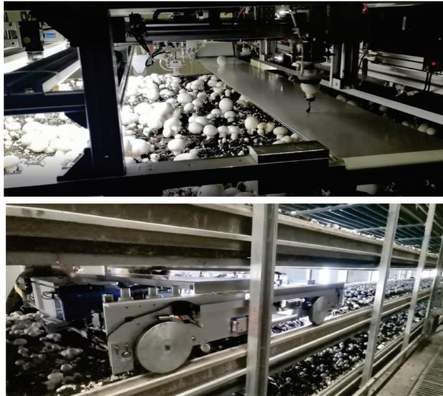
Figure 13. The multiarm intelligent harvesting robot working in the multistory shelf trays in the factory environment.
