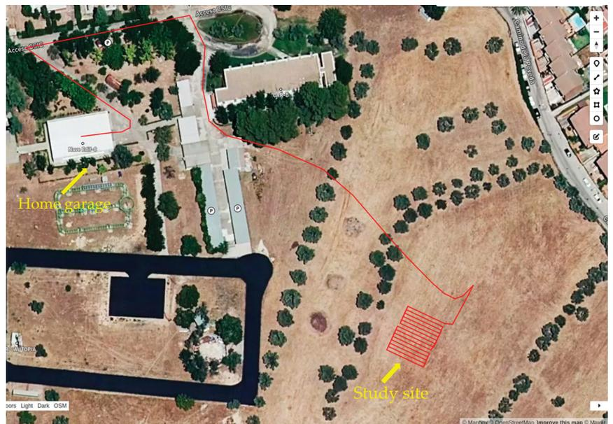
**Figure 7.** Robot's path from the home garage to the study site. The planner provides the mission for covering the study site.
