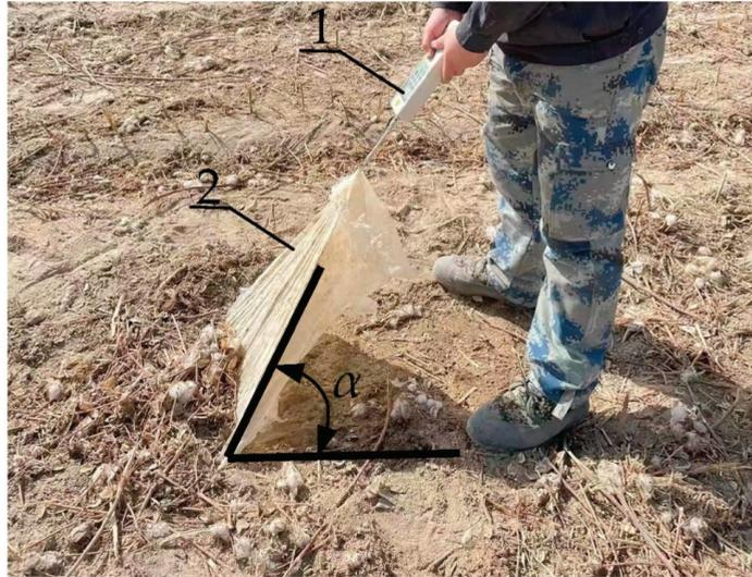
**Figure 6.** Test field on curl-up force in film collecting: 1—HP-50 type Digital Display Pull and Push Strength Calculator, 2—film.
