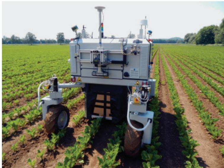
**Figure 2.** Acquisition process of the Sugar Beets dataset using the BoniRob terrestrial robot developed by Bosch DeepField Robotics [15]. BoniRob is equipped with four wheels that can be steered independently of each other, allowing flexible movement and navigation on rough terrain.
