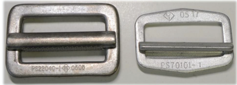
Figure 2. Selected buckles for the frame preparation to create the measuring load cell.
