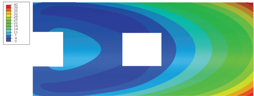
Figure 19. Deformation of the outer face sheet in millimetres on the lattice/PCM model for combined thermal and pressure loading. Cutouts represent the areas with local effects around the nodal constraints that were ignored in stress evaluations.
