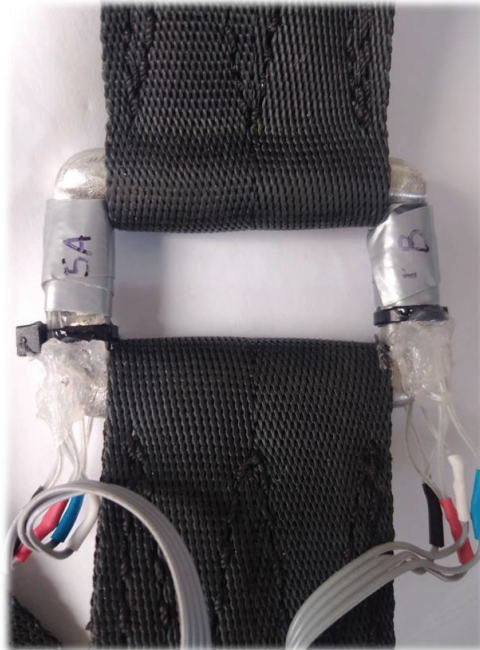
Figure 4. Final load cell manufactured on PS22040-1 baseplate sewn into structure.
