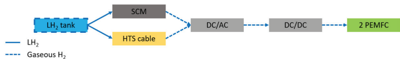
Figure 7. Hydrogen flow from the fuel tanks to the fuel-cell system; full line representing liquid hydrogen and dotted line representing gaseous hydrogen.
