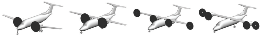
Figure 3. Redesign of a Beechcraft 1900D (left), modified redesign (centre-left), as well as non-optimized PT2025 (centre-right) and optimized PT2025opt (right) versions of the partial turboelectric concept aircraft.
