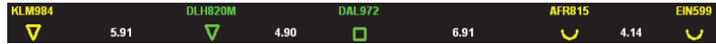
Figure 6. The CSVT. The symbols mark the positions of aircraft (triangle), ghosts (square) and TargetWindows (semicircle). The labels' colours represent the aircraft's weight classes (yellow: medium; green: heavy), and the white numbers between the labels indicate the current separation between them.
