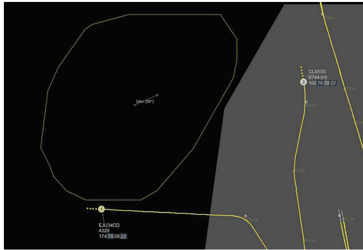
Figure 18. The dark color scheme with convective zones displayed as bordered areas. Malpensa traffic mix from 11 May 2019 with weather from 11 May 2019 and the WRF-RUC nowcast model.
