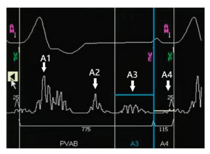
Figure 2. Schematic illustration and explanation of the key atrial sensing parameters. The top signal shows the electrocardiogram; the bottom signal shows the accelerometer signal.
