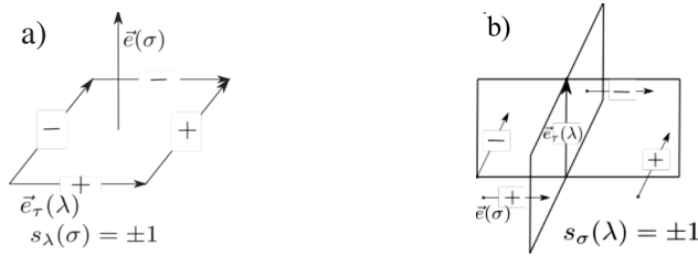
Figure 2. Circular matching of oriented normals to faces \sigma on the left and tangents along mesh edges \lambda on the right. The sign function s_\lambda(\sigma) = \pm 1 (a) takes values according to whether the orientation of the edge \vec{e}_\tau(\lambda) coincides with the direction of rotation about the normal \vec{e}(\sigma) . The sign function s_\sigma(\lambda) = \pm 1 (b) is defined similarly, but the contour is made up of oriented face normals \vec{e}(\sigma) , and the rotation is around the tangent along the edges \vec{e}_\tau(\lambda) .
