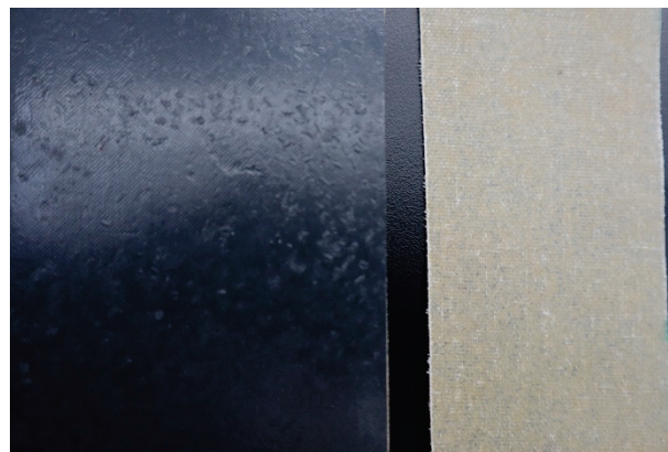
Figure 1. Pictures of the ABS (left) and GF prepreg (right) sheets used to manufacture distinct sandwich composite panels.
