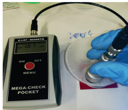
Figure 4. Thickness measurement on solvent-casted polymer-BP films.
