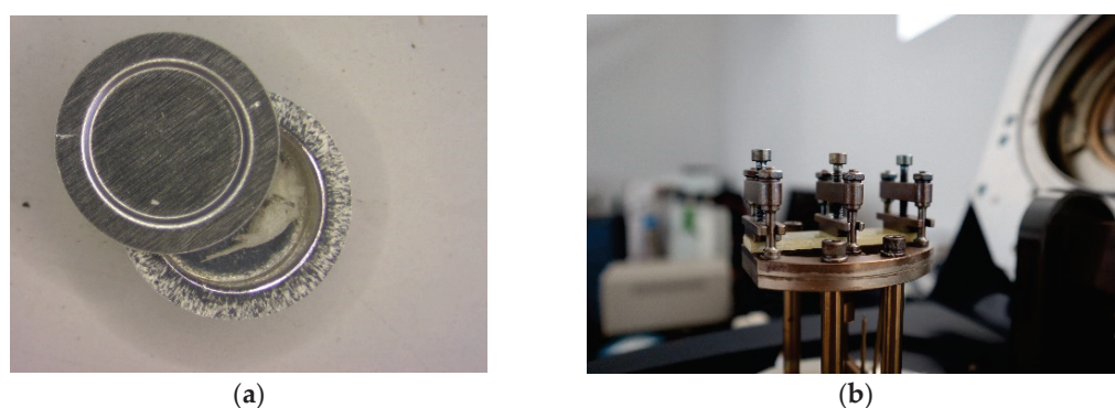
Figure 2. Pictures of representative tests of: (a) samples in the aluminum pan before hermetic close and test by differential scanning calorimetry (DSC), (b) specimen of glass fiber before testing in dynamic mechanical analysis (DMA).
