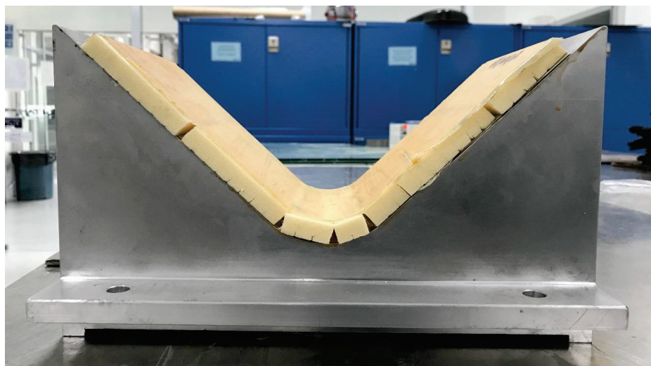
Figure 5. Picture corresponding to the gridding foam specimen placement in the V-shaped mold before the preheated process.
