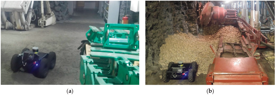
Figure 4. Underground inspection scenarios: (a) smooth terrain before accident; (b) rough terrain after accident.
