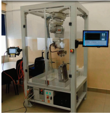
Figure 1. Robotic station for controlling the thickness of OGV airfoils.
