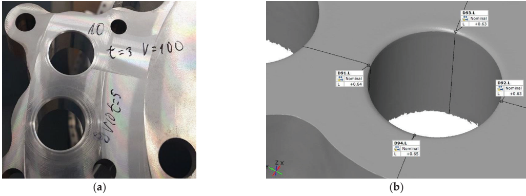
Figure 20. Deburred ADT gearbox housing: (a) block section; (b) measuring the repeatability of the radius.
