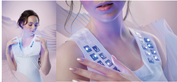
Figure 2. Diffuse and mask layer with parametric patterns (left) and Undergarment with Embroidered conductor tracks and bonded PCBs (right).
