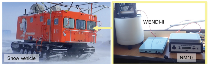
Figure 2. A photograph of the snow vehicle (left) and the portable neutron monitor (WENDI-II) connected to an exclusive data logger (NM10) (right) originally made for mobile use. The neutron monitor was placed near the front window inside the snow vehicle.
