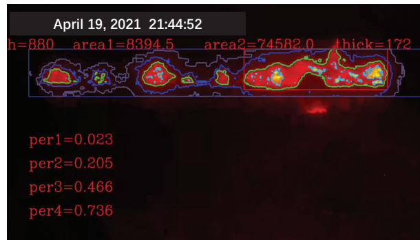
Figure 16. Video feature extraction diagram of the red layer at the end of the sintering machine.
