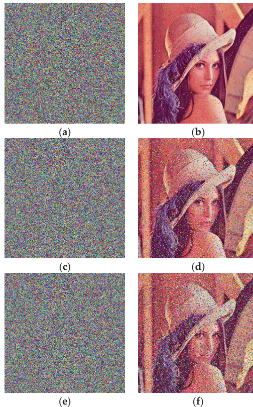
Figure 11. Noise experiment adding noise intensity of (a) 0.02, (b) 0.12, and (c) 0.2 after the encrypted image, and (d–f) is its corresponding decryption image.
