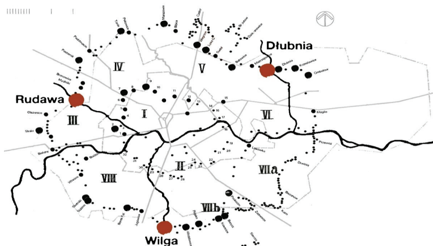
Figure 1. Diagrammatic plan of the Krakow Fortress with the locations of previously unknown impoundment structures marked in dark brown, accompanied by the boundaries of defensive areas I through VIII.
