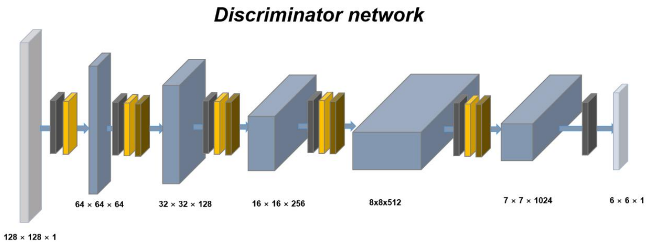
Figure 3. Model architecture of the discriminator for generating synthetic MR images from lumbar spine CT. The generator used a PatchGAN discriminator. Each number of the feature maps is the width, height, and channels of the feature map. The layers for networks were constructed by the color boxes. MR, magnetic resonance; CT, computed tomography.
