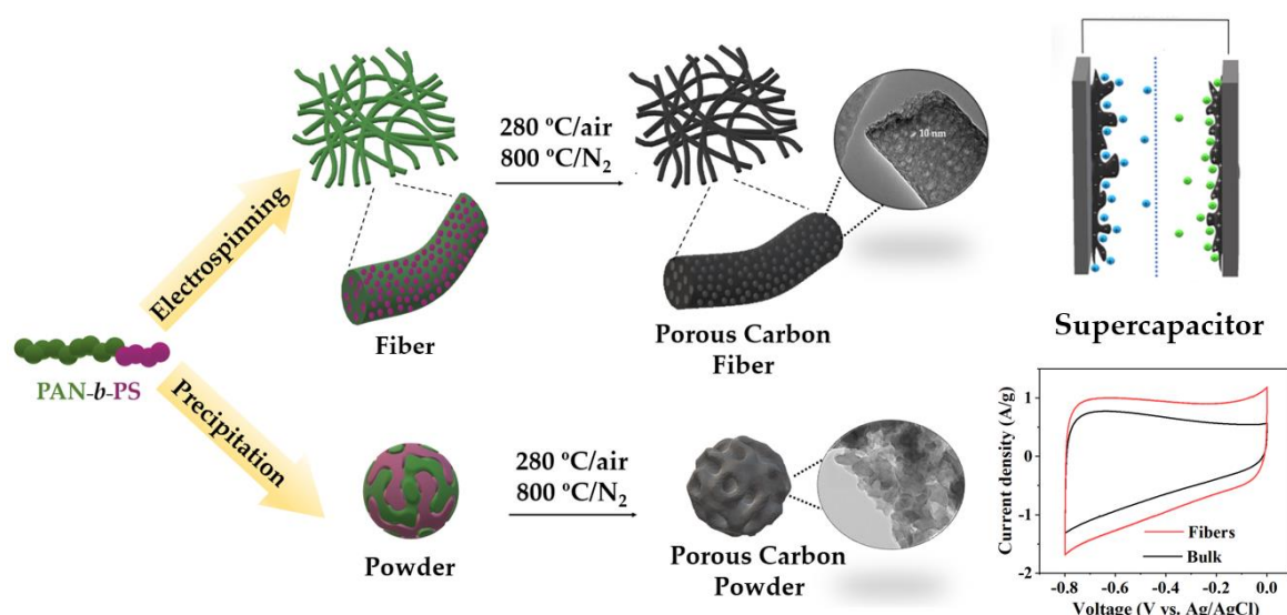
Scheme 1. Preparation scheme of porous carbon fibers and powders, from PAN– b –PS copolymer template for use as supercapacitor electrode materials.
