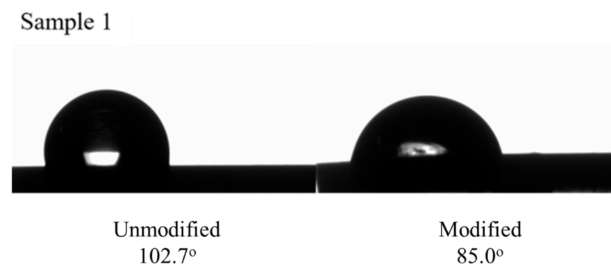
Figure 4. Images of water contact angles corresponding to the \text{PS-}b\text{-PB}_{1,2}\text{-}b\text{-PDMS} terpolymer (sample 1). The left image corresponds to the unmodified, pristine terpolymer, and the right image to the finally modified case.
