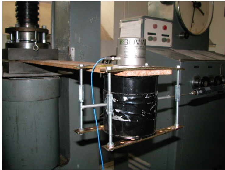
Figure 9. Cantilever beam experimental tests scheme. The vibrodyne is on the bottom while the accelerometer is on the top side of the free end.
