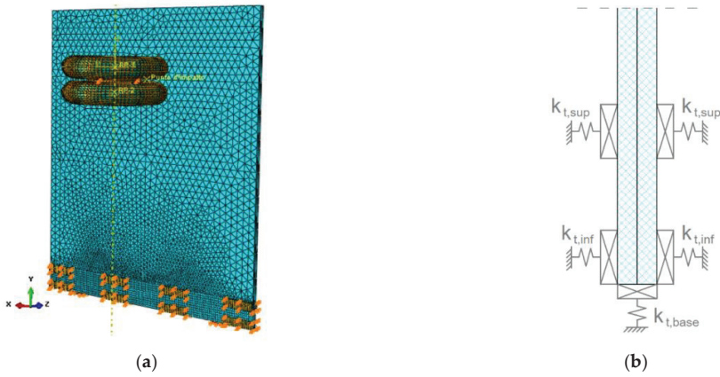
Figure 7. SM1 simplified model: (a) model concept and 3D assembly (axonometric view from ABAQUS), with (b) the reference mechanical system (cross-section) and evidence of lumped equivalent springs.
