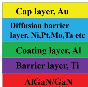
Figure 5. Schematic structure of metal stacks used for forming ohmic contact to AlGaIn/GaN HEMT.
