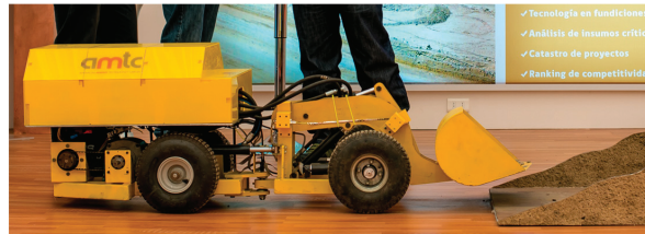
Figure 12. 1:5 scaled LHD built for testing and validation.
