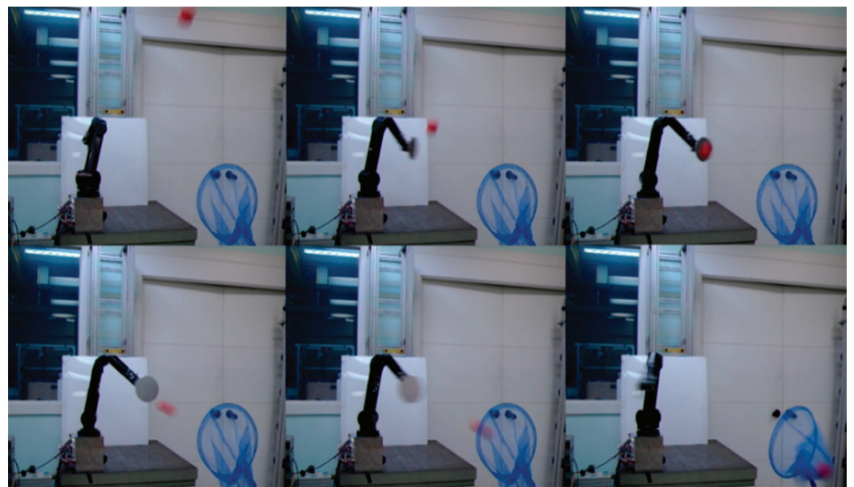
Figure 14. Successive snapshots of batting task (sequence is horizontal to vertical).
