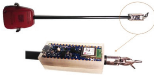
Figure 5. Complete prototype of the first version of the detection device connected to the EndoWrist tool of dVRK system.
