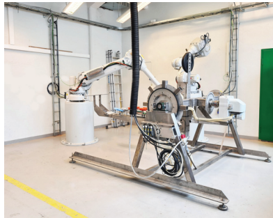
Figure 2. Carcass handling unit in the RoButcher laboratory.
