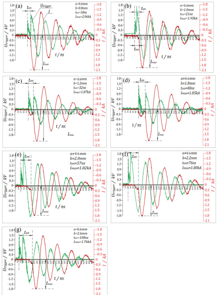
Figure 9. The tested waveform of switch conduction performance (a) b = 0.8 mm, (b) b = 1.0 mm, (c) b = 1.2 mm, (d) b = 1.8 mm, (e) b = 2.0 mm, (f) b = 2.2 mm, (g) b = 2.6 mm.
