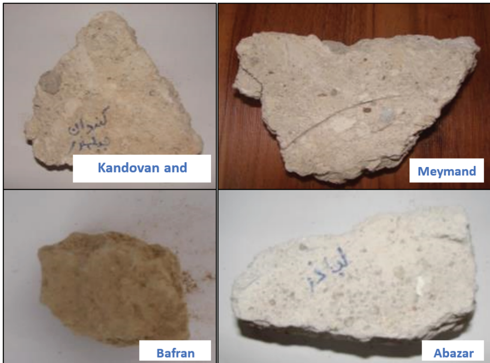
Figure 8. Pumice stones found in Meymand, Kandovan and Abazar and their difference with the dense sediment found in Bafran.
