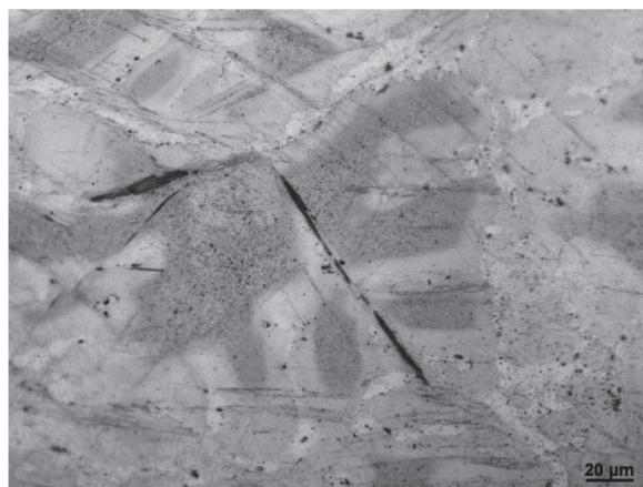
Figure 17. The crack in the P6 specimen.
