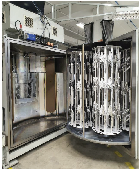
Figure 7. A photo of the fully loaded chamber with samples mounted on planetaria.
