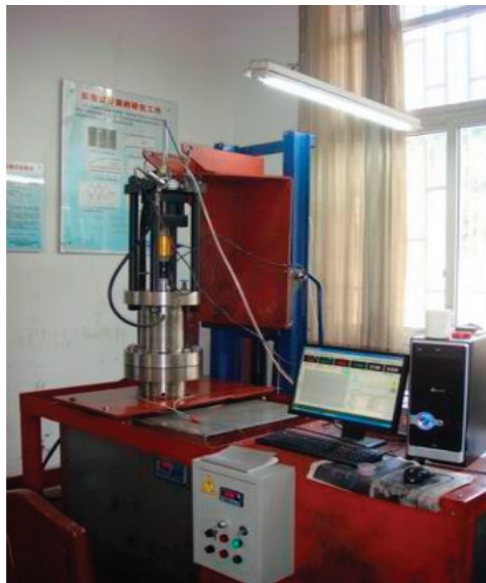
Figure 2. The triaxial servo-controlled seepage equipment for thermofluid–solid coupling of coal containing methane.
