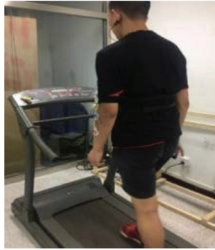
Figure 1. A treadmill used to simulate the intensity of a miner's working.
