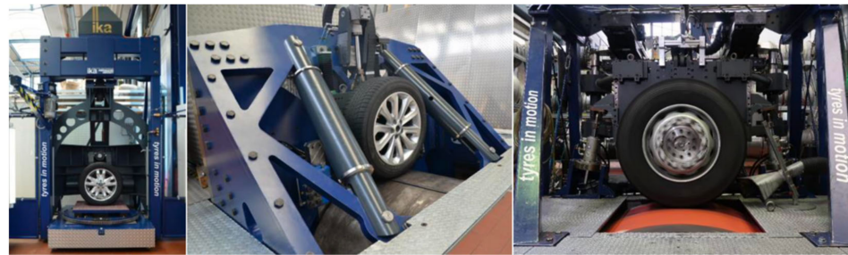
Figure 12. Tire test rigs used for experimental investigation of tire properties to parameterize and validate the FTire tire model.
