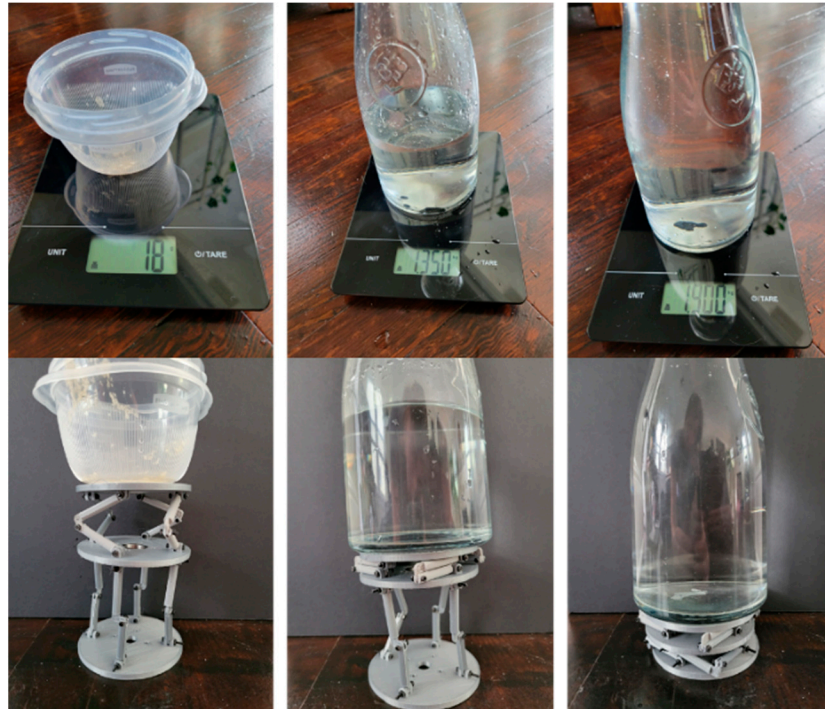
Figure 20. Weight of load applied to a two-section structure with the top section half folded initially.
