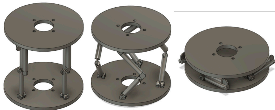
Figure 14. The three images from left to right show the folding of a single Kirigami section.
