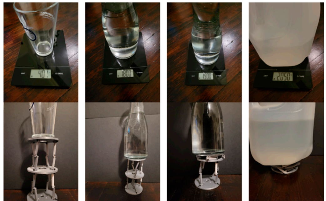
Figure 19. Weight of load applied to a fully extended two-section structure.
