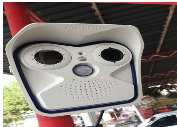
Figure 2. Thermal imaging camera which was used in the experiment.
