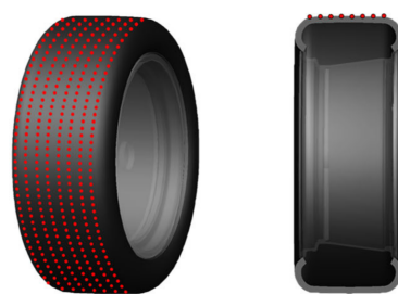
Figure 11. Example illustration of the arrangement of brush-type contact elements (tread blocks) in lines (tread strips) on the tire belt of the FTire model.
