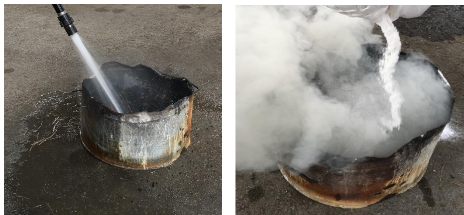
Figure 6. Brushwood fire suppressions with water and solid boron-based fire suppressant.
