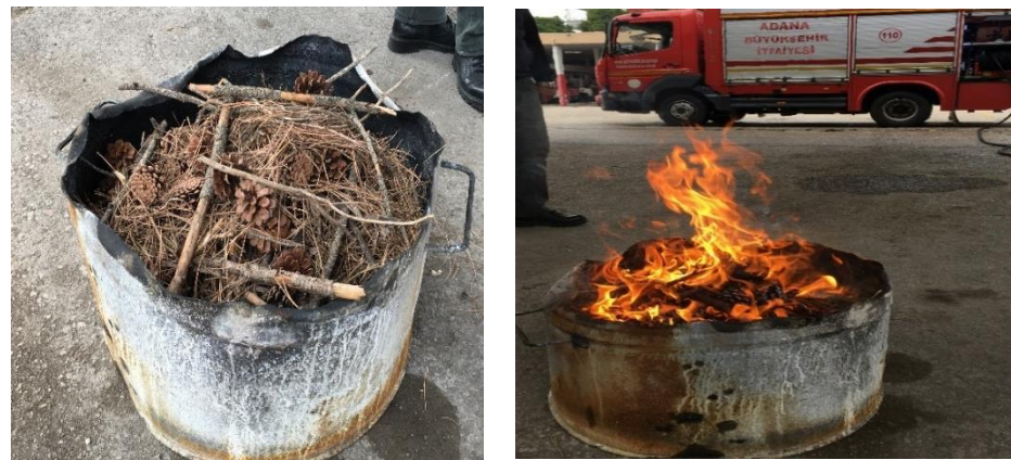
Figure 5. Brushwood fire setup.
