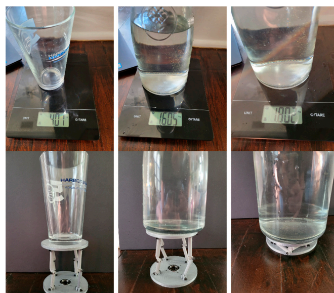
Figure 18. Weight of load applied to the revolute structure and resulting structural deformations. The photos in the top row show the actual load and those in the bottom row show the responses to the structure deformations.
