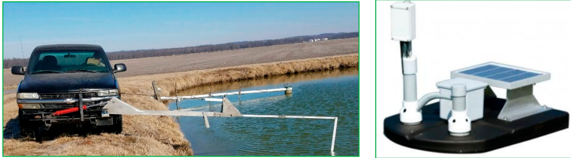
Figure 2. (a) The typical truck-based boom sensor system. (b) The “top-of-the-line” in situ buoy system from In-Situ Inc [11].
