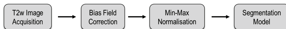
Figure 1. The image pre-processing for T2-weighted images. After acquisition, bias field correction was applied using the N4 algorithm to correct for the magnetic field inhomogeneity. The images were then normalized using the min–max approach before entering the segmentation network.
