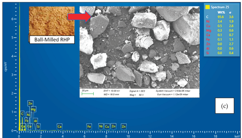
Figure 1. FESEM image and their corresponding EDS spectrum for (a) CBP (b) WSP (c) RHP.
