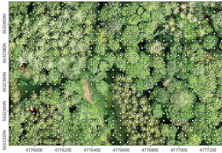
Figure 5. Orthophoto of the grid application region recorded on 2 July 2020. White dots mark points where photos were taken during the automated 5 m × 5 m grid flight. Coordinates are given in UTM zone 32N.
