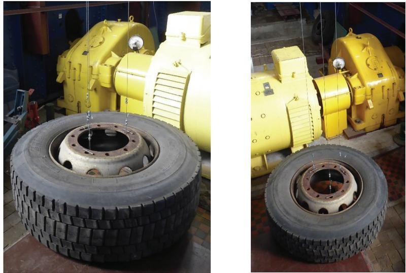
**Figure 5.** Wheel mounted on the stand for determining the mass moment of inertia.
