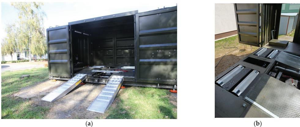
**Figure 1.** A mobile dynamometer device: (a) front view, (b) view of the interior of the dynamometer (authors' source).
