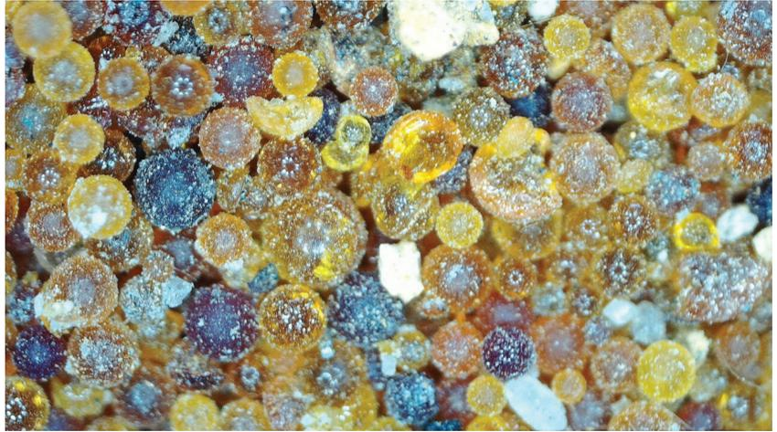
**Figure 3.** Optical microscopy of ion exchange resin spill, observed in situ. To the naked eye, this was indistinguishable from finely ground ore sand, but its real nature became clear under the microscope (see Figure 2) which also enabled a particle size distribution and morphology to be characterised.
