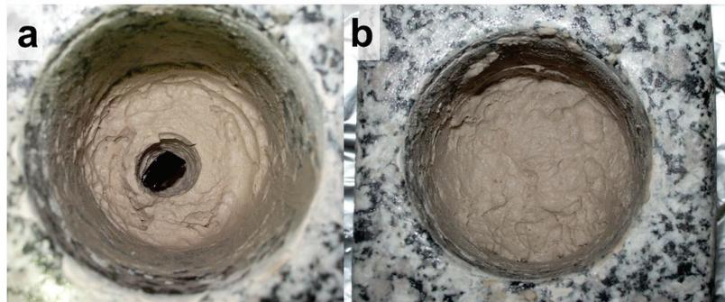
**Figure 2.** Preparation of the experiment: (a)—the Pu-doped borosilicate glass surrounded by wet bentonite inside the granite container; (b)—view after sealing filling with bentonite.
