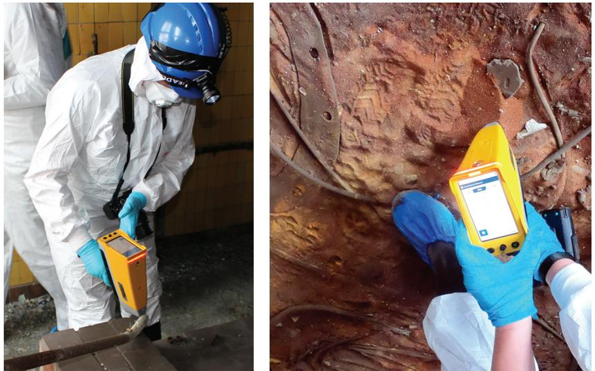
**Figure 2.** A portable XRF analyser (type: Olympus Vanta) used for in situ nuclear industrial archaeology of samples in a legacy uranium ore processing facility. **(Left)** Nuclear industrial archaeology of contamination on construction material. **(Right)** Nuclear industrial archaeology of a spill of ionic exchange resins.
