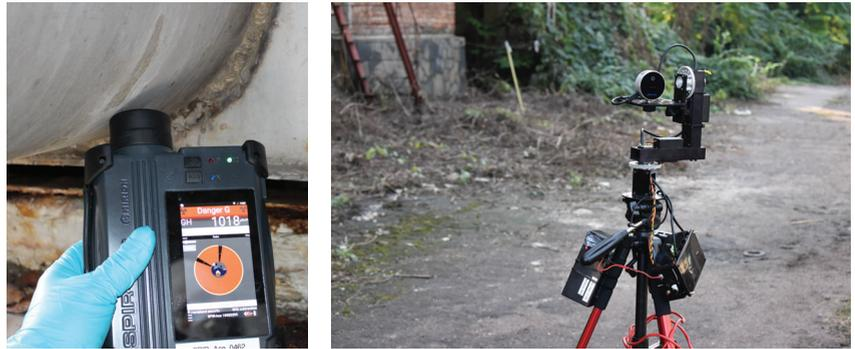
**Figure 1.** Gamma spectroscopy in field-deployed nuclear industrial archaeology. (Left) a portable NaI(Tl) gamma spectrometer of type Mirion SPIR-Ace [52] used to measure gamma radiation dose rates in excess of  $1.0 \text{ mSv h}^{-1}$  on the outside of a pipe connecting a mixer–settler tank in a legacy uranium ore processing facility. (Right) a collimated gamma spectrometer [53] mounted on a pan-tilt unit and suspended on a tripod to map contamination in an industrial environment [51].
