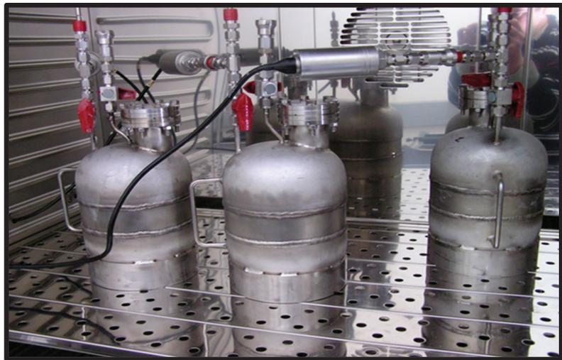
**Figure 2.** View of the long-term batch experiment on the Boom Clay rock ships at 80 °C.
