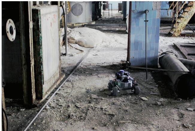
**Figure 8.** Deploying a remote-controlled wheeled ground vehicle equipped with gamma spectrometer and neutron detector in an environment with radioactive contamination.
