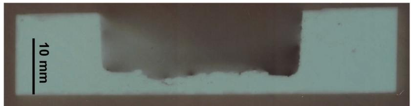
**Figure 8.** Autoradiography (2 months exposure) of the granite sample from the bottom of experimental granite container: cross section of lower part. Black rectangle appears due to  $\alpha$ -particles reaching the film through air gap.
