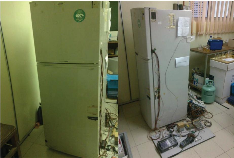
Figure 1. Domestic refrigerator test-rig.
