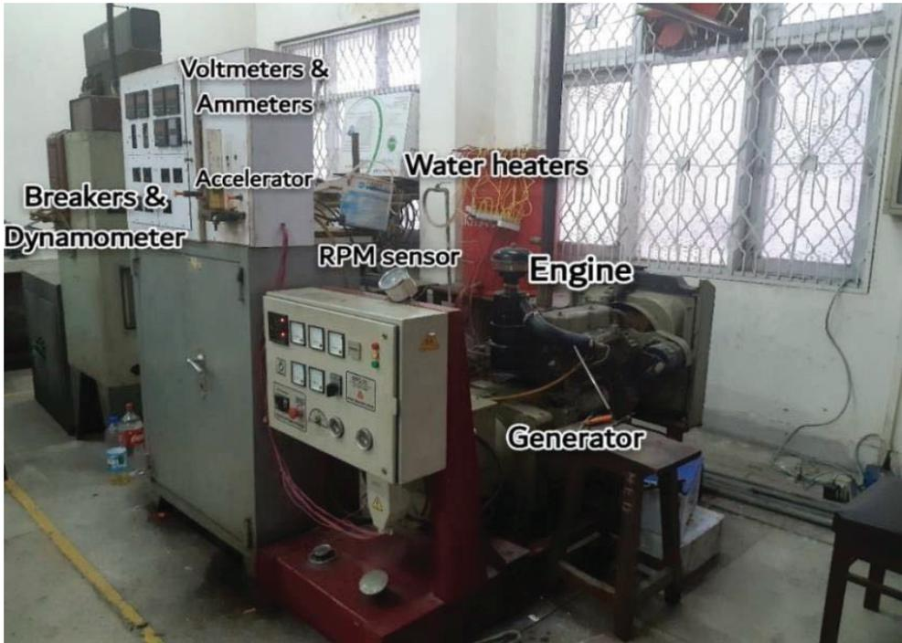
Figure 2. Experimental setup.
